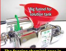
The fogging chemical goes in the larger tank. Use the big funnel to fill the tank.
