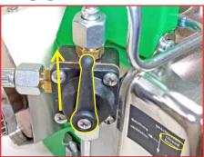
Before starting, make sure the Solution Tap Valve is CLOSED (handle points up).
