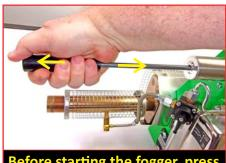
Before starting the fogger, press the Starter Button and cycle the Air Pump a few times to build pressure in the tanks.
