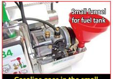
Gasoline goes in the small tank at the rear of the fogger. Use the small funnel to fill the tank and reduce spills.
