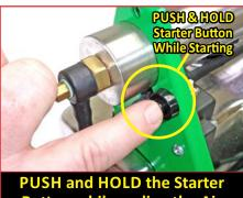
PUSH and HOLD the Starter Button while cycling the Air Pump. Hold Starter Button for 10 seconds after fogger starts.
